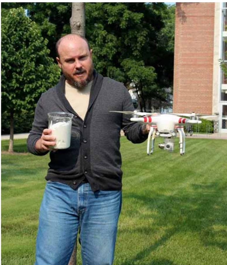
UAVs can be retrofitted to transport pheromone-loaded “wax soup” (SPLAT<sup>®</sup>) across the marsh, depositing the wax according to a pre-set flight plan. This research represents a public-private collaboration between the Steffan (Entomology) and Luck (Biological Systems Engineering) laboratories at UW-Madison, as well as the private company, ISCA Technologies, Inc. (Riverside, CA). Photo courtesy Joan Fischer, University of Wisconsin.
