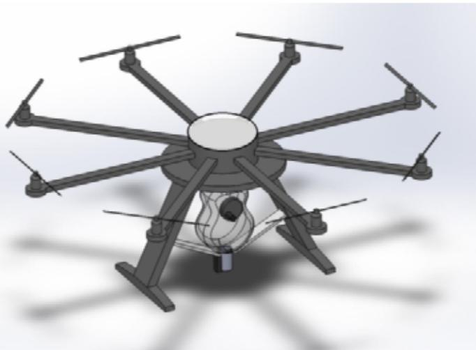
Early design of a retrofitted UAV. This prototype involves an octocopter platform with GPS-navigation system. Artwork courtesy of Cullen Winebar, University of Wisconsin.
